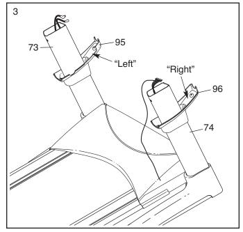
4. With the help of a second person, hold the console assembly near the Uprights (73, 74).
